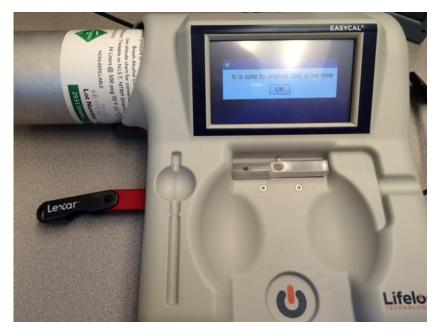
Take the USB drive off and transfer the data into a computer/lap top
