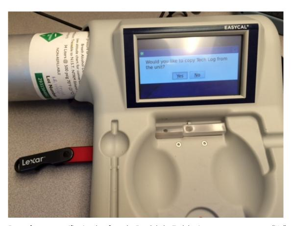
For performance verification data from the EasyCal, the Tech log is not necessary so press "No"
