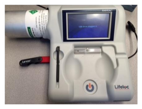
Plug in a USB thumb drive into the EasyCal. This will automatically be recognized by the unit with a message "USB Drive plugged in"
